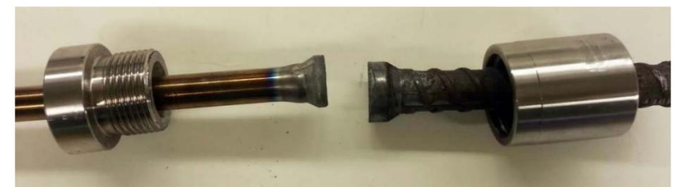
SMA to steel rebar coupler unassembled.
