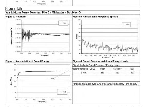
Figure 15: Waveform analysis of Pile 5 sound pressure levels without (a) and with (b) bubbles, midwater.
