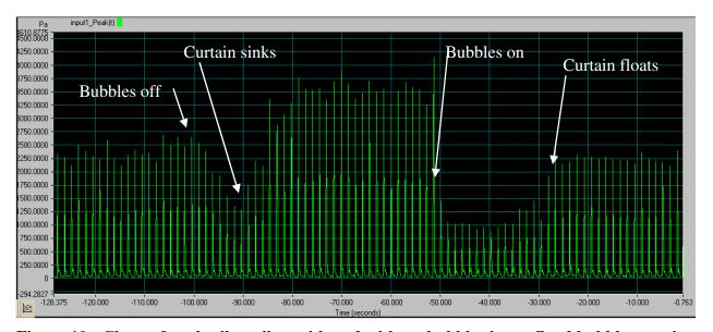
Figure 10: Chart of peak pile strikes with and without bubbles in confined bubble curtain.
