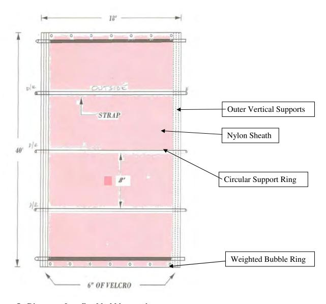
Figure 5: Diagram of confined bubble curtain.
