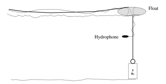
Figure 4: Diagram of hydrophone deployment configuration.
