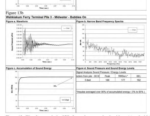
Figure 13: Waveform analysis of Pile 3 sound pressure levels without (a) and with Bubbles (b), midwater.
