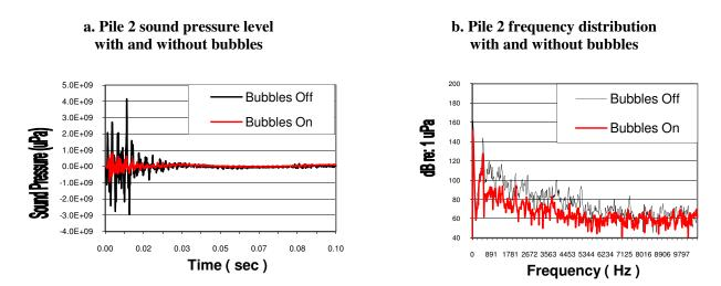
Figure 6: Waveforms and frequency spectral analysis for pile 2 with bubbles on and off.
