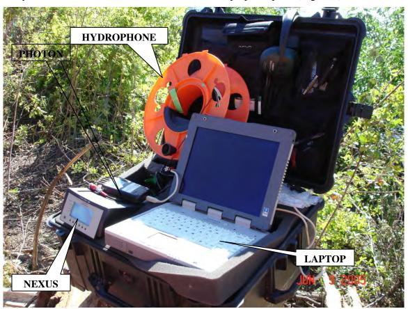
Figure 3: Near field acoustical monitoring equipment
