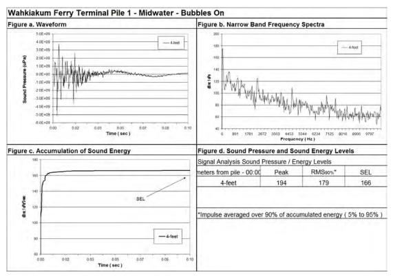
Figure 11: Waveform analysis of Pile 1 sound pressure levels with mitigation, 4 feet water depth.
