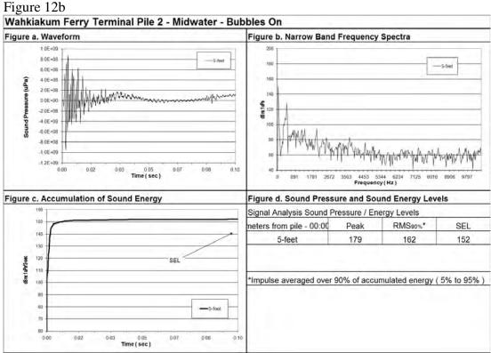
Figure 12: Waveform analysis of Pile 2 sound pressure levels with bubbles off (a) and bubbles on (b).
