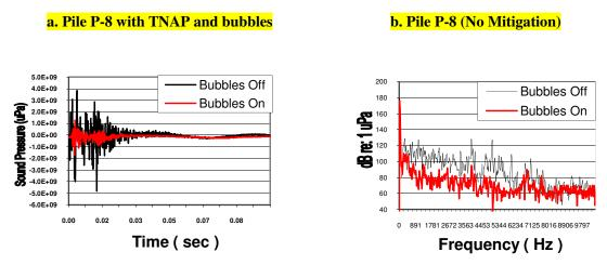
Figure 9: Waveforms and frequency spectral analysis for pile P-8 using the TNAP.
