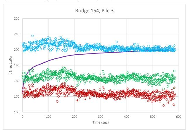
Figure 18: Time history plot of individual pile strikes for Bridge 154, Pile 3
