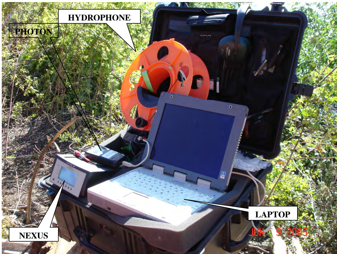
Figure 3: Near field acoustical monitoring equipment
