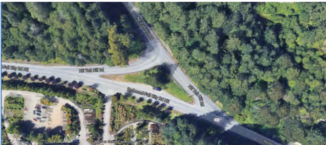
An aerial view of the Y-shaped intersection of Northeast Tolt Hill Road and SR 202, Tolt Hill splits into two for easier turns to and from SR 202 in either direction.
