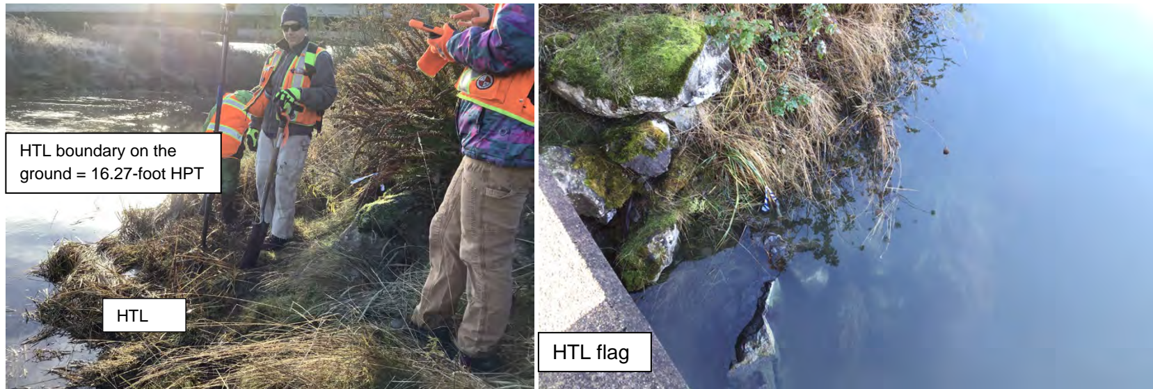
(Left) HTL delineation on McAllister Creek on December 15, 2022. (Right) HTL verification during king tide event at on McAllister Creek on December 28, 2022. Additional HTL observation points were recorded within the study area and are presented below.
